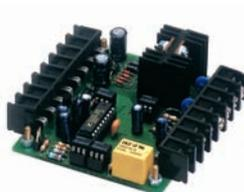
**The SYNC900 synchronizer module interfaces between the Control Panel and the HS900.**
