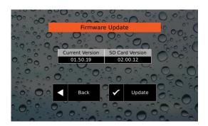
4. Press Update: the update may take some time (about 2 min, a progress bar shows the proceeding of the upgrade), no more action can be done before Firmware upgrade will be completed; once it is complete, the keypad returns to the Advanced Menu.
