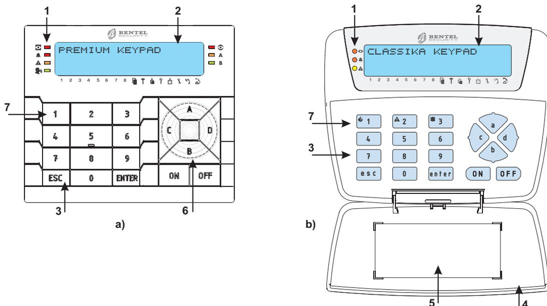
**Figure 1** - a) PREMIUM LCD Keypad, b) CLASSIKA LCD Keypad.
