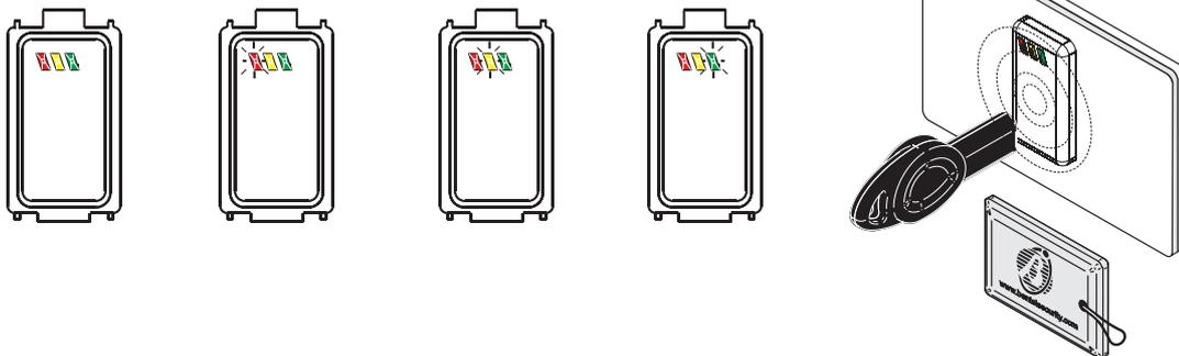
**Figure 4** Disarm/Arm/Stop Alarms from ECLIPSE2 reader.
