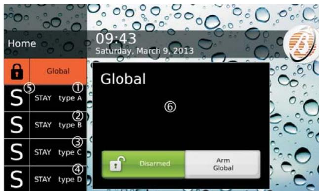
**Figure 28** Arming by the Touch Keypad: labels 1, 2, 3 and 4 can be customised, as explained in the text; the corresponding Special arming initial letter will be put in position 5; the description assigned to the arming selected will appear in window 6, as explained in the text.
